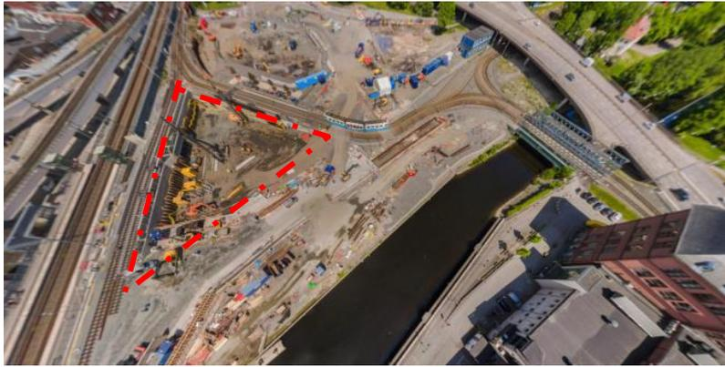
*Figure 2 Aerial photo of the triangular shaped piling site bounded by railway bridge, river and tram lines*
