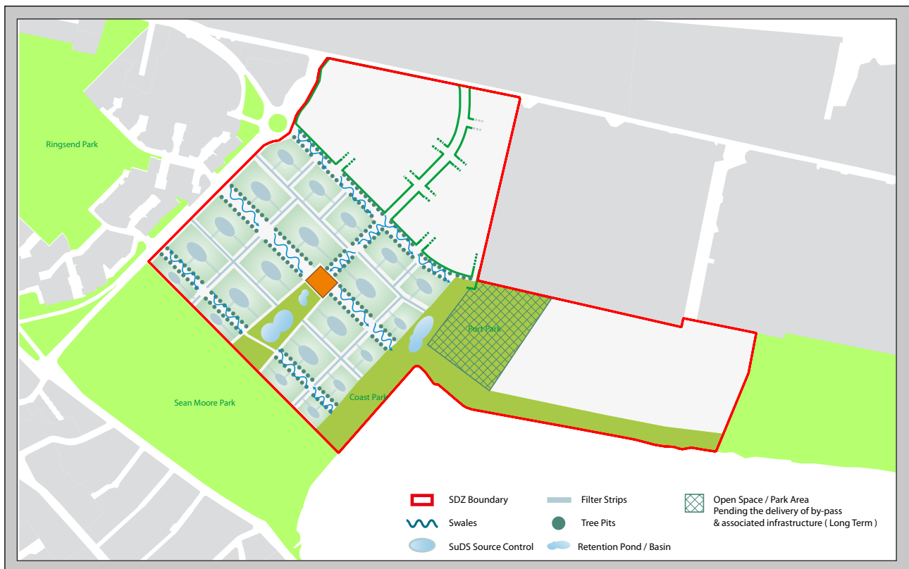
Figure 1.2: Extract from the Poolbeg West SDZ Planning Scheme (Dublin City Council) illustrating the surface water drainage network which includes an integrated public realm and public open space network to provide high quality and attractive 'green and blue' corridors to enhance local amenity, ecology and biodiversity.
