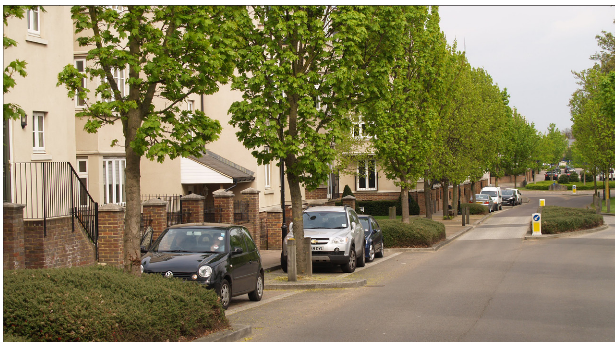
Figure 3.1: Extract from DMURS (figure 4.28) illustrating the integration of planting into the design of a street to increase visual amenity, support biodiversity and calm traffic.
