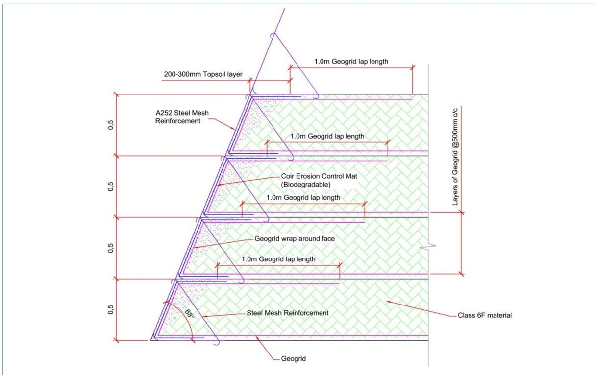
Figure 4 - Embankment construction details
